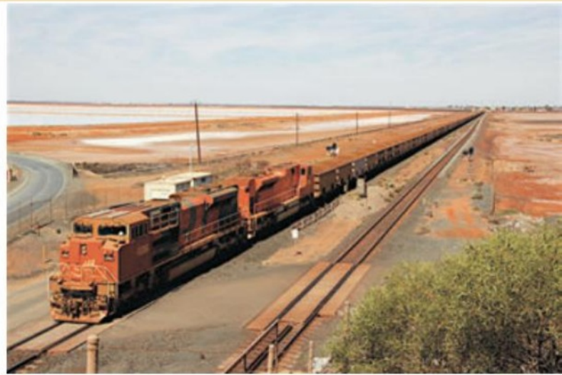
3.44 A BHP Billiton iron ore train arrives in Port Hedland after its 426 kilometre journey from Newman. Like all the BHP trains, this train is 2.6 kilometres long, and consists of 4 diesel locomotives, 248 ore cars and one driver. Each ore car holds 130 to 138 tonnes of iron ore, and the train has a total load of 33,000 tonnes. The train travels at 65 kilometres per hour, so the journey from Newman to Port Hedland takes about seven hours.
