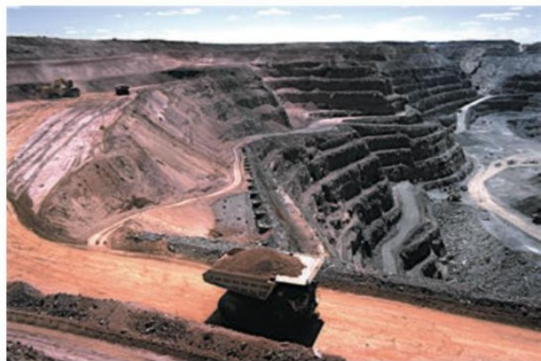
3.32 Another view of the Fimiston Open Pit in the desert of Kalgoorlie, Western Australia. Large trucks transport the gold ore for processing. The pit has a rectangular shape, and is 3.5 kilometres long, 1.5 kilometres wide and 570 metres deep.
