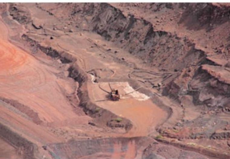
3.38 One of the challenges of deep open-cut mining is keeping the mine dry as the pit fills with water from surrounding aquifers. This pump in the bottom of the Mount Whaleback mine pumps water into the channel that runs through the bottom of the mine.
