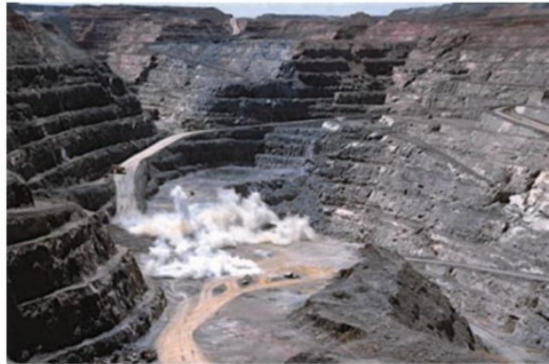
3.31 An open-cut gold mine is blasted to break up rocks at the bottom of quarry, sending dust into the atmosphere. This is the Fimiston Open Pit, also known colloquially as the 'Super Pit', in Kalgoorlie, Western Australia. It is Australia's largest open cut gold mine, and it is surrounded by desert.
