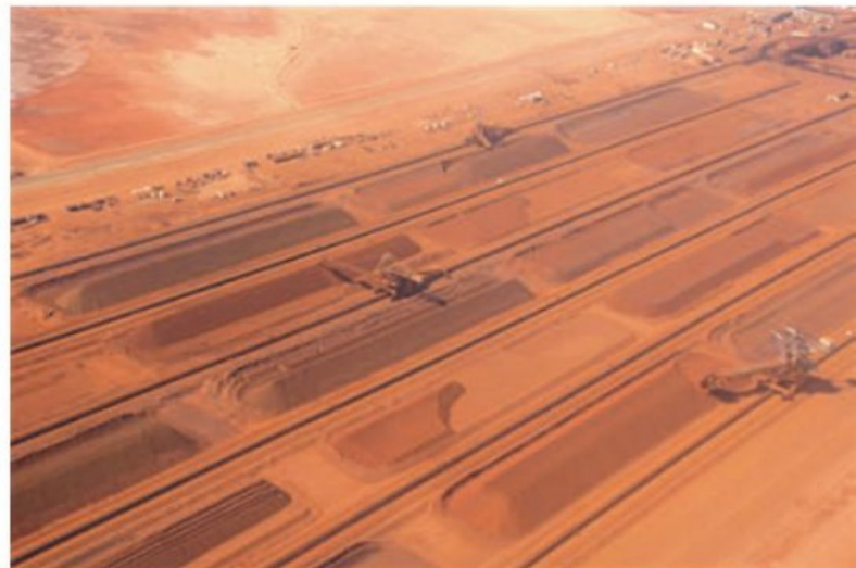
3.45 When the iron ore arrives at the port, it is unloaded from the trains and held in stockpiles before loading onto ships for export. This shows part of the Fortescue Metals Group stockpile at Port Hedland.
