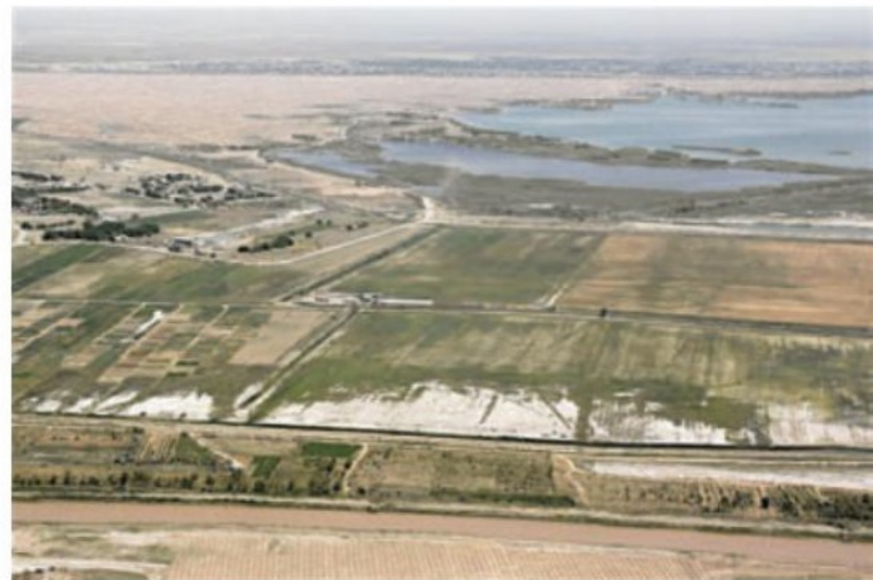
3.7 The white areas on these fields is salt, brought to the surface by poor irrigation practices. Excessive quantities of water have been pumped from the Karakum Canal (the brown channel in the foreground) onto these fields near Ashgabat at the southern fringe of the Karakum Desert in Turkmenistan. The excessively wet soil has freed the salts to rise to the surface, destroying the land for agriculture.
